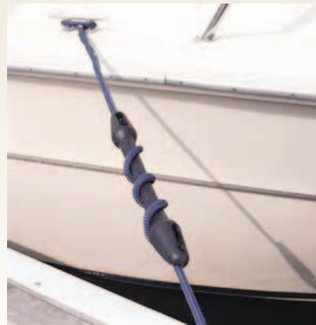
Here are two kinds of snubbers to use when dock ties are vertical. The snubbers provide slack needed to offset movement, particularly in winter storms.
