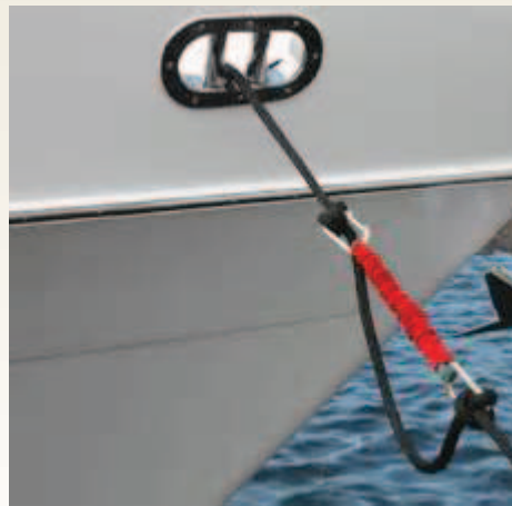
Here are two kinds of snubbers to use when dock ties are vertical. The snubbers provide slack needed to offset movement, particularly in winter storms.
